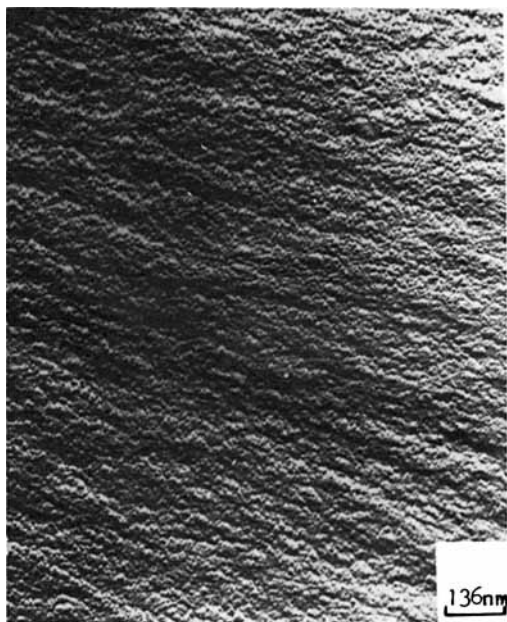
Fig. 3. Transmission electron micrograph of a fracture surface replica of dry TGDDM/DDS epoxy resin. Magnification 73,000 \times . Note the inhomogeneous structure of the fracture surface.
